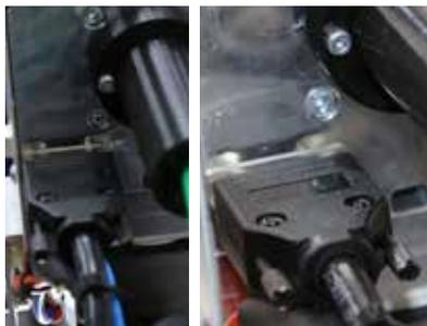
6. Connect the black laser cable to the port on the back of the laser head at the top of the articulating arm.
