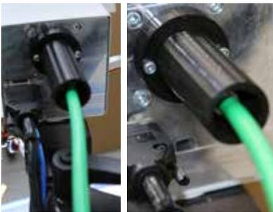
5. Connect the green laser cable to the port on the back of the laser head
