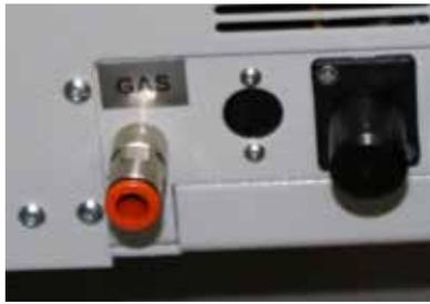
11. If using shielding gas, connect the gas tube into the gas port on the back of the power supply.
