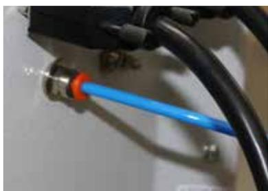
7. Connect the blue air cable to the air port on the back of the laser head at the top of the articulating arm.
