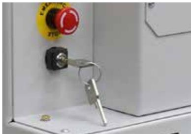
14. Insert the key on the front of the power supply and turn it clockwise to allow the welder to function.
