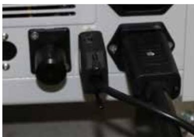
8. Connect the foot pedal cable to the foot pedal port on the back of the power supply.
