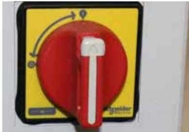
13. Turn the welder power switch on the back of the welder clockwise to turn on the welder.
