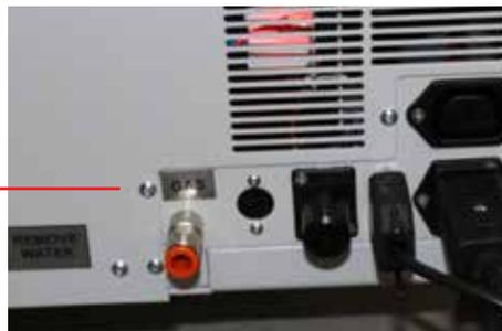
**Picture 6: Protection gas connection and air connection**
